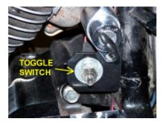
Slide Heat Shrink over back of toggle switch to switch plate, and gently apply heat until heat shrink is snug over all parts.
