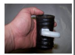
direction (do not re-install filler hose until you have attached the 1/2" fill hose to the 'L' connector in later step).
