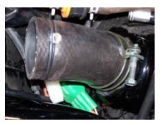
Attach 'L' connector making sure to place one washer on each side of the filler hose before tightening. 'L' Connector should be facing out the left side of the trike with a slight rearward
