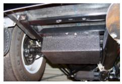
5) Installing Fuel Pump: (Use stainless clamps provided for all hose connections)
