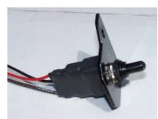
Unbolt ignition switch, slide Switch Plate between ignition switch and frame; re-secure ignition switch and toggle assembly in place.
