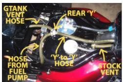
Connect 25" hose from fuel pump outlet to Rear 'Y' connector, keeping hose inside of right lower frame rail, then up between main tank and intersection of right
